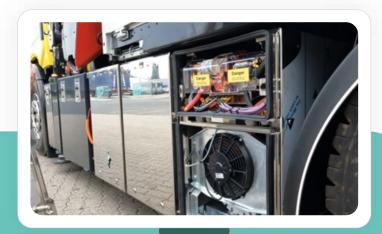
Discover Blue Pac Vertical Original, an innovative and ecofriendly electric crane drive solution. With energy-efficient ePTO technology, emissions and noise are reduced, while operating costs are lowered compared to diesel operation. The slim, customizable modules blend seamlessly with the truck's design, and thanks to standardized battery and motor modules from ETP Power Electronics, installation is simple and smooth. A sustainable solution for the future of the transportation industry.
